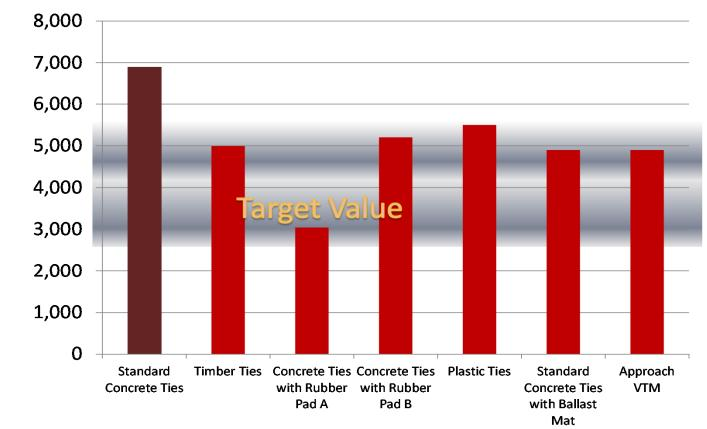
Average VTM of the test spans at FAST with Plastic Ties and Concrete Ties with a ballast mat (VTM from previous test are shown)
